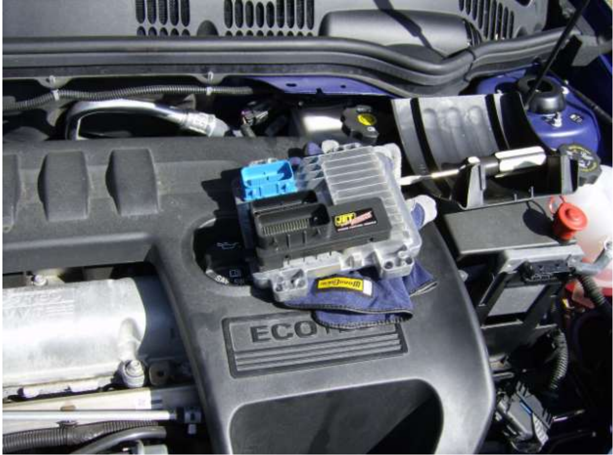
Jet Performance Product's GM Performance Module 10708 (Stage 1) in ECU
