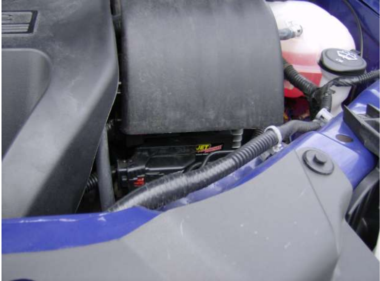
Jet GPM peaking out from under ECU cover
